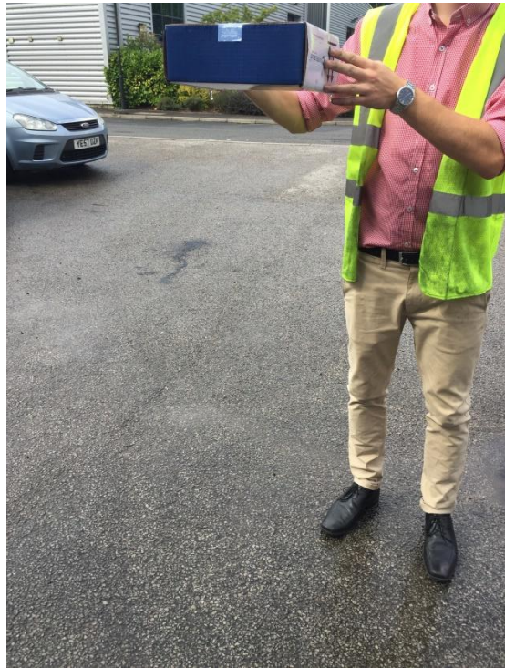
P4 system being dropped after simulated rainfall
