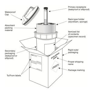
**Figure 9.** Example of the triple packaging system for the packing and labelling of Category B infectious substances (Figure kindly provided by IATA, Montreal, Canada)
